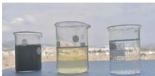
Picture 2: Comparison of original sample (left), with iron electrodes (in the middle) in 3 hours electrocution and with BDD and Ti/Pt electrodes in 2 hours electro-oxidation (right)
