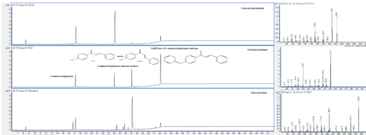
Figure 2. Comparison of the Total Ion Chromatograms (TIC) of the crude reaction mixture of 4-aminoacetophenone and benzaldehyde using conventional, grinding techniques and sonication, and the mass spectra of the main products
