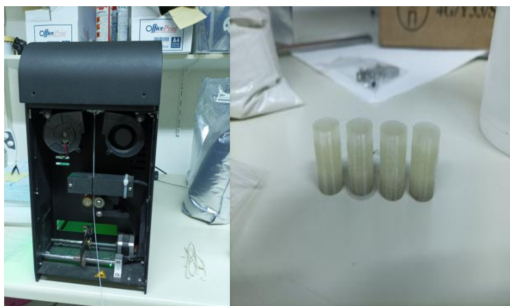
Figure 1 The extruder (on the left) and the produced specimens (on the right).
